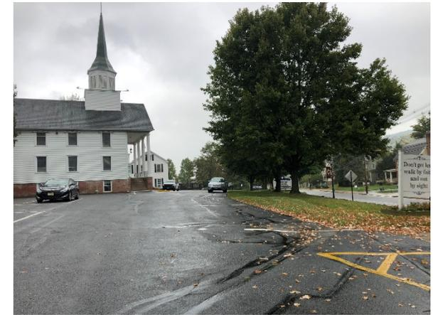
Parking spaces in the parking lot to the northeast of the building can be converted to porous pavement to capture and infiltrate stormwater runoff from the parking lot. A rain garden can be installed in the turfgrass area near the entrance of the building to capture, treat, and infiltrate stormwater runoff from the roof. A preliminary soil assessment suggests that more soil testing would be required before determining the soil's suitability for green infrastructure.
